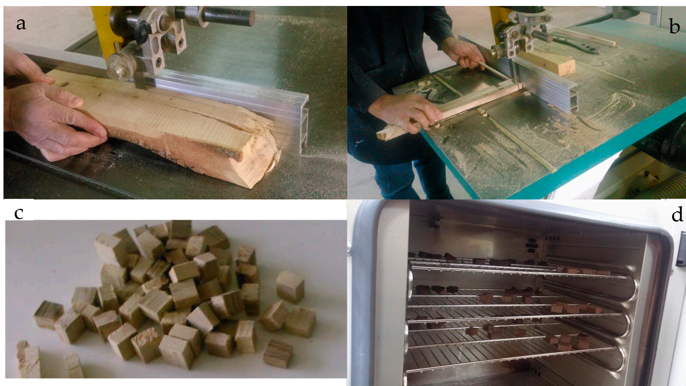
Figure S3. Cutting process of the different type of woods (a) and (b) at cubs of dimensions 2.0 \times 2.0 \times 1.0 cm (c). Toasting process of wood cubes (d).
