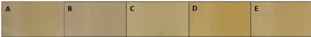
Figure 4. Photographs of the pressed grape juice treated with different electric field strengths. (A) Grape juice from untreated grapes. (B) Grape juice from grapes treated with 2 kV/cm. (C) Grape juice from grapes treated with 3 kV/cm. (D) Grape juice from grapes treated with 4.5 kV/cm. (E) Grape juice from grapes treated with 6 kV/cm.
