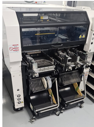
Figure 1. Overview of the SMT pick-and-place machine setup, showing the reel feeders and operational area.
