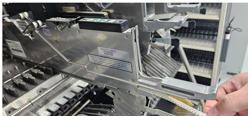
Figure 2. Reel being positioned in the feeder slot during the exchange process.
