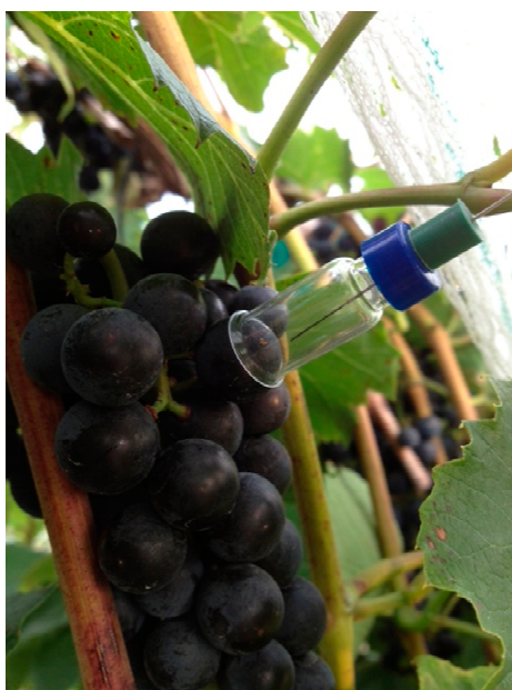
Figure 1. Biogenic volatiles were collected by solid-phase microextraction (SPME) released from grape skin. A glass vial was modified for vacuum-assisted SPME of volatile organic compounds (VOC)s from a single grape. The vacuum was created with a syringe prior to SPME, so the vial was adhering to the skin and sealing headspace for SPME.
