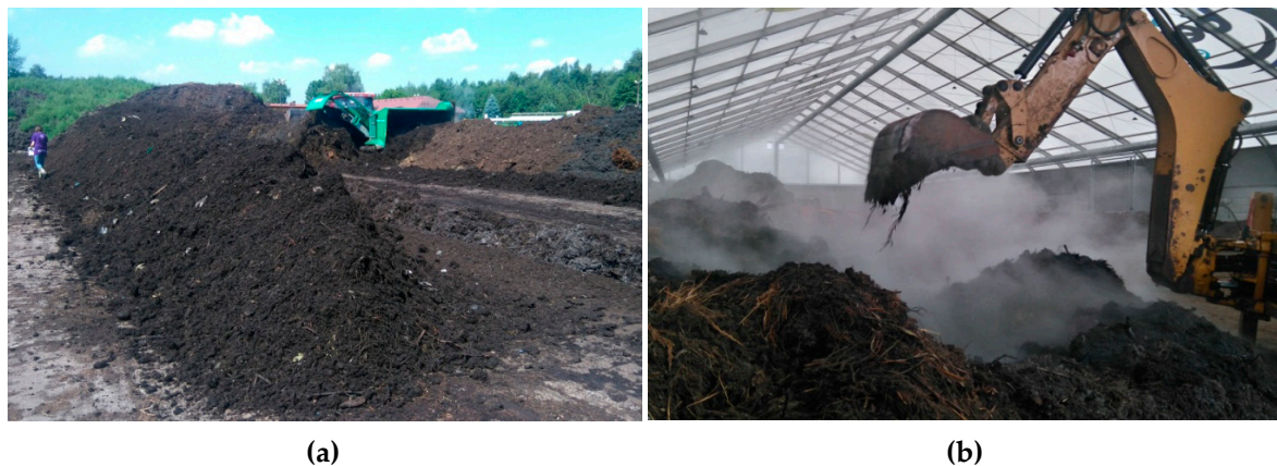
Figure 2. Turning of the compost material (a) pile A2 outdoors; (b) pile A5 inside a composting hall.
