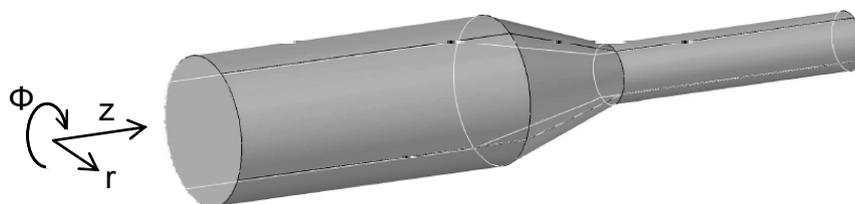
Figure 1. Diameter reduction in a pipeline.
