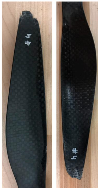
Figure 9. Broken propeller #4.
