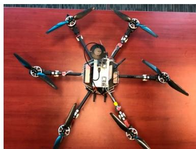
**Figure 1.** Tarot-RC 690 Hexacopter Unmanned Aerial System (UAS).
