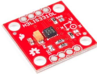
**Figure 10.** ST H3LIS331DL three-axis accelerometer.
