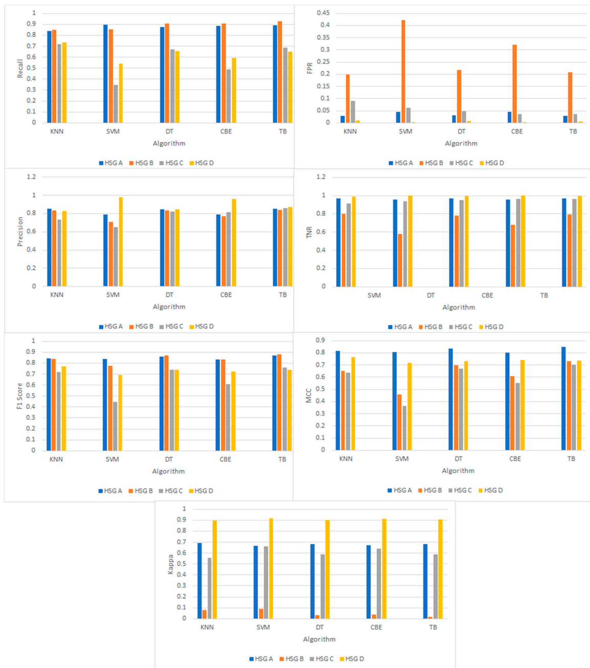
Figure 3. A graphical representation of per-class performance metrics for kNN, SVM-Gaussian Kernel, Decision Trees and Ensemble Learning Algorithms (CBE and TB).
