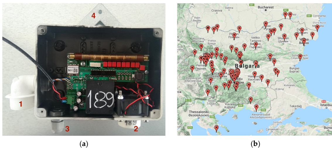
Figure 1. Network outlook: (a) Each device consists of an input (1) and output (2) valve, cable fitting (3) and assembly part (4); (b) current coverage map of Bulgaria and Greece.
