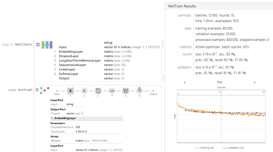
Figure 12. The architecture of the “GloVe + LSTM” deep neural network and its training results.
