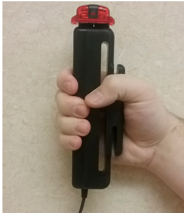
Figure 1. Image for how the dynamometer was securely attached to the accelerometer with velcro.
