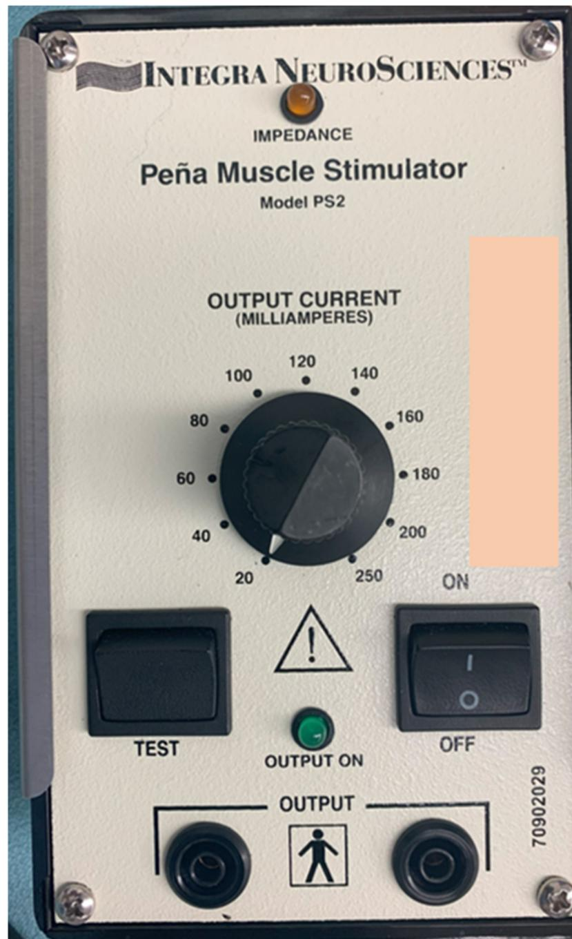
**Figure 4.** The stimulator/power supply component of the Peña stimulator. The output of the device can be adjusted to achieve the best stimulation at the lowest output.
