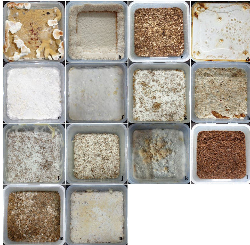
Figure 2. Topography of the mycelial mat generated from the Polyporales species. (a) Ganoderma lucidum , (b) G. applanatum , (c) Elfvigia applanate , (d) Fomitella fraxinea , (e) Formitopsis pinicola -JF, (f) F. pinicola -KCTC, (g) F. rosea , (h) Trametes versicolor , (i) T. hirsuta , (j) T. suaveolens , (k) Wolfiporia extensa , (l) Microporus affinis , (m) Bjerkandera adusta , (n) Postia balsamea .
