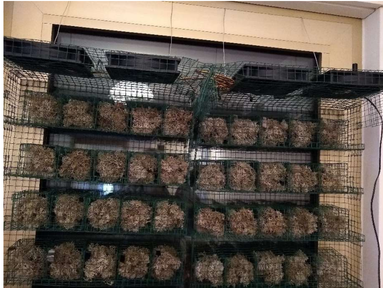
Figure S2. Pictures of the custom-built wire mesh cages containing each one approximately 4.5 g of lichens. Cages were installed in a vertical structure hanging from a window with fans on top of the samples to promote drying after watering treatments.
