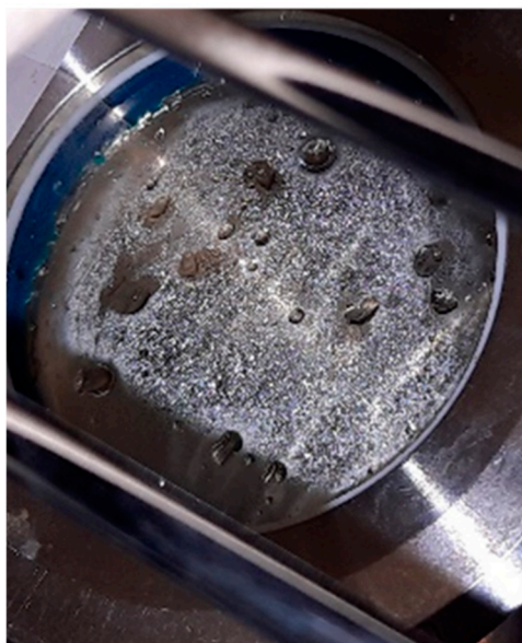
Figure S12: Used polycondensation vessel as reactor unit, with condensation media on sight glass.
