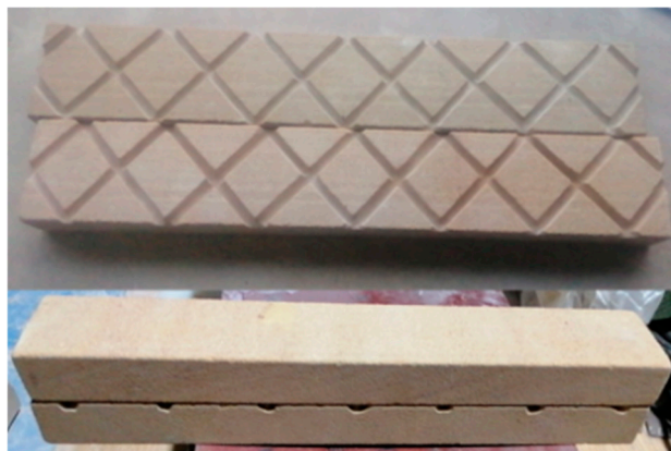
Figure 11. Design and physical image of complex fracture core model.
