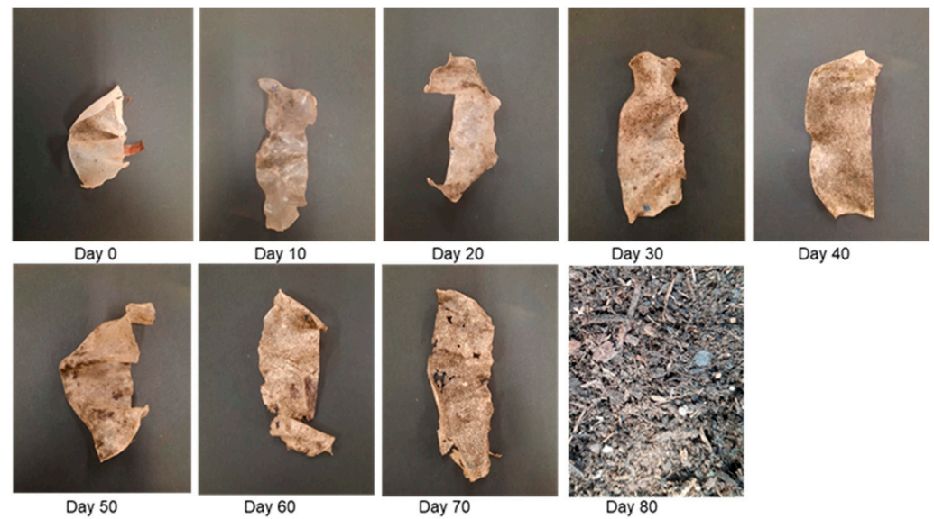
Figure 8. Morphological changes in soil cover samples during their soil burial degradation: visual images.
