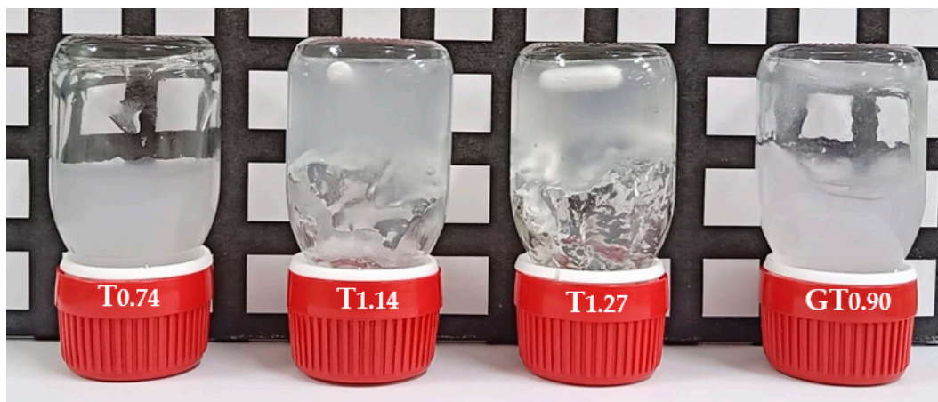
Figure 1. Digital photos of 0.80 wt.% aqueous suspensions of T 0.74 , T 1.14 , T 1.27 , and Cat. CNFs. The photos were taken at room temperature.
