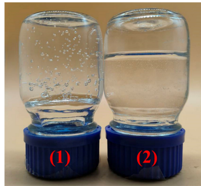
Figure 8. The picture of degradable gel: (1) after gelation, (2) after degradation.
