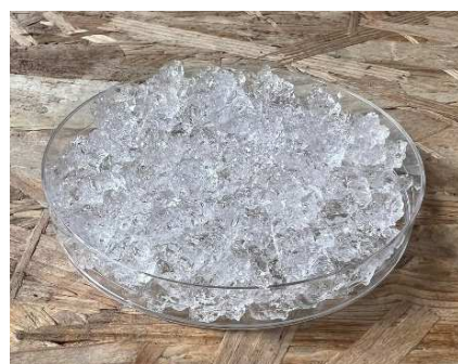
Figure 19. Photograph of the coarse hydrogel sample exposed to microwave radiation and for 480 min again placed in a water bath.
