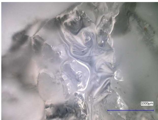
(a) Microscope 100×, fine hydrogel after EMW followed by wetting
