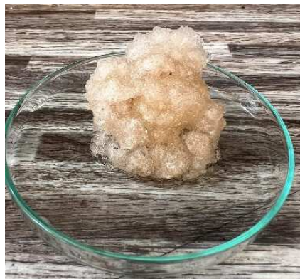
Figure 18. Photograph of the coarse hydrogel sample exposed to microwave radiation and for 5 min placed again in a water bath.
