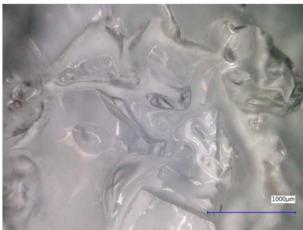
(a) Microscope 100×, coarse hydrogel after EMW followed by wetting
