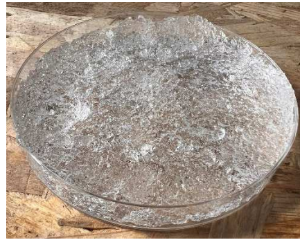
Figure 21. Photograph of the fine hydrogel sample exposed to microwave radiation and for 480 min again placed in a water bath.
