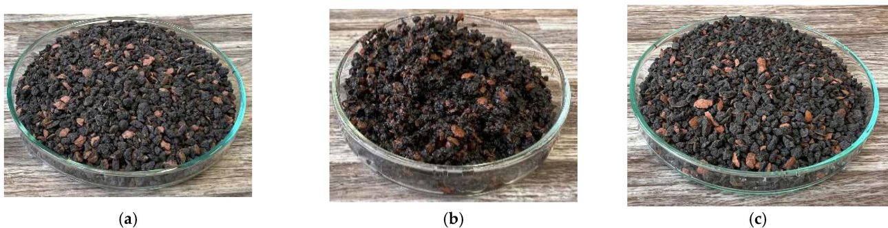
Figure 25. Photographs of the ceramsite sample during the experiment. (a) Photograph of ceramsite sample before wetting. (b) Photograph of ceramsite sample after wetting. (c) Photograph of ceramsite sample after exposure to microwave radiation.
