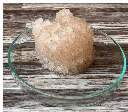
Figure 20. Photograph of the fine hydrogel sample exposed to microwave radiation and for 5 min placed again in a water bath.
