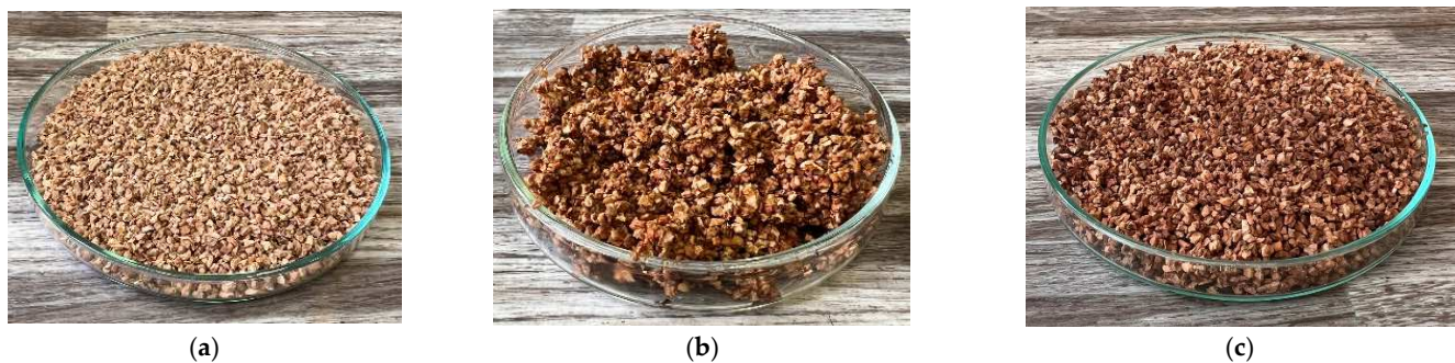
Figure 24. Photographs of the coarse cork sample during the experiment. (a) Photograph of cork sample 2 before wetting. (b) Photograph of cork sample 2 after wetting. (c) Photograph of cork sample 2 after exposure to microwave radiation.
