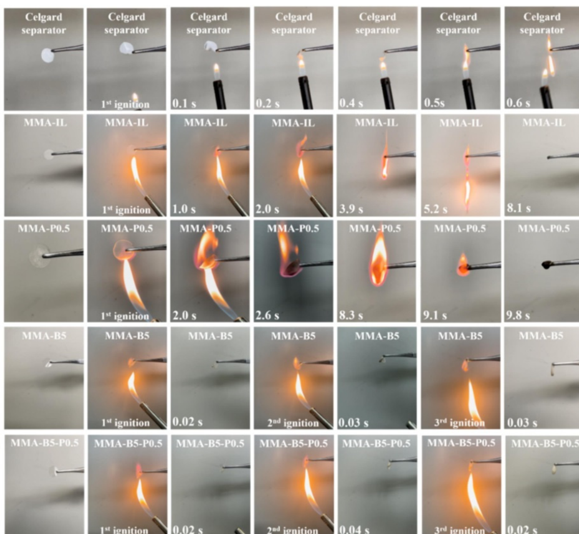
Figure 14. Fire resistance tests for the Celgard separator and GPE films, reproduced with permission from ref. [102], Elsevier.
