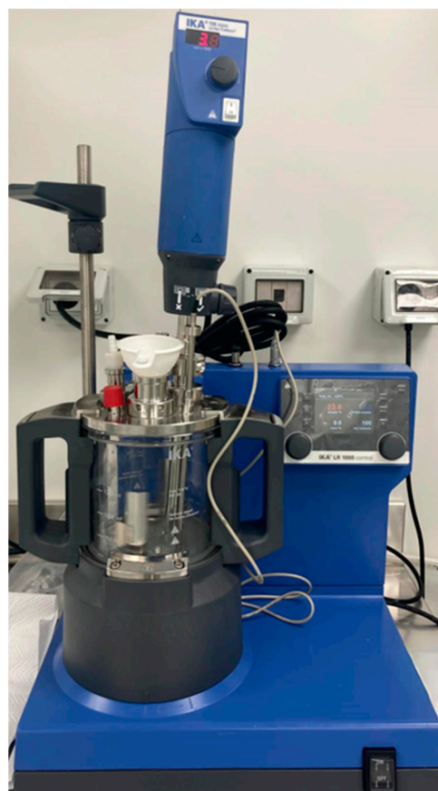
Figure S6. The IKA® LR 1000 reactor (Staufen, Germany) equipped with the T25 Ultra-Turrax dispersing tool (IKA, Staufen, Germany) used for the preparation of niaprazine-loaded XG gels.
