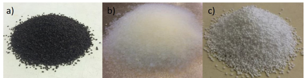
Figure 8. Lightweight aggregates used in the study: (a) regranulated expanded cork (GEC); (b) hydrophobic silica aerogel (SA); and (c) expanded polystyrene (EPS).
