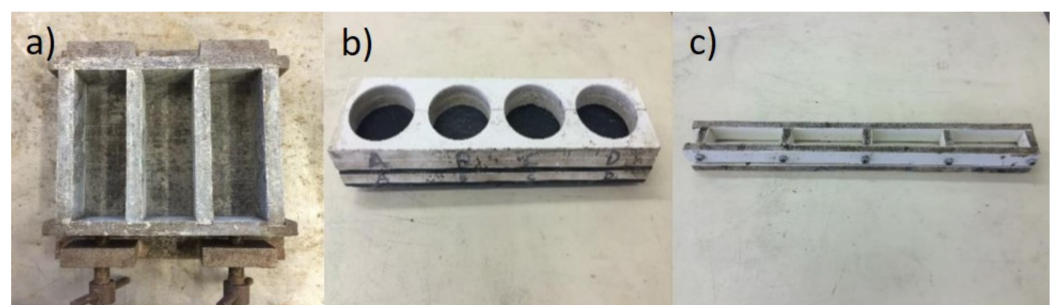
Figure 9. Moulds used in production of specimens: (a) standard specimens ( 40 \times 40 \times 160 mm 3 ); (b) thermal conductivity specimens (60 mm diameter and 20 mm thickness); (c) small-size specimens ( 20 \times 20 \times 80 mm 3 ).
