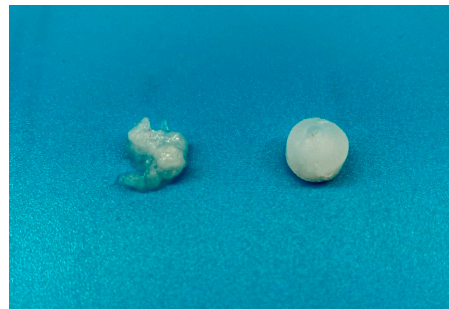
Figure 8. GG 24 (on the right) and GG 8 (on the left) ionotropic crosslinked hydrogels after 1 week of incubation at 37 °C in DPBS pH 7.4.
