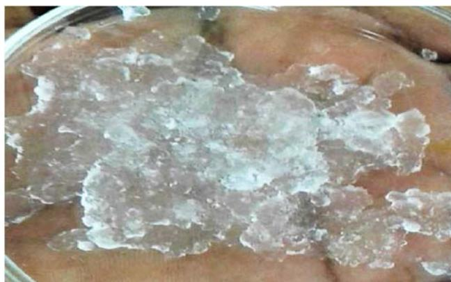
**Figure 3.** Cellulose-co-AMPS hydrogel after absorption of water.
