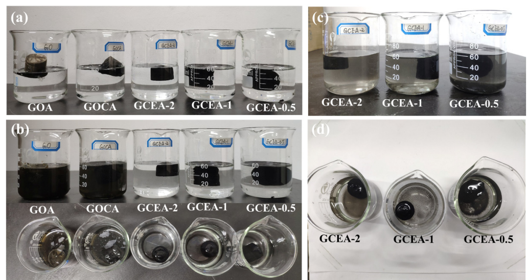
Figure 5. The digital images of GOA, GOCA, and GCEA immersed in water, (a) 0 min, (b) ultrasonic treatment for 1 min (side and top view), (c,d) the GCEA in ultrasonic treatment for 30 min (Color figure can be viewed online).
