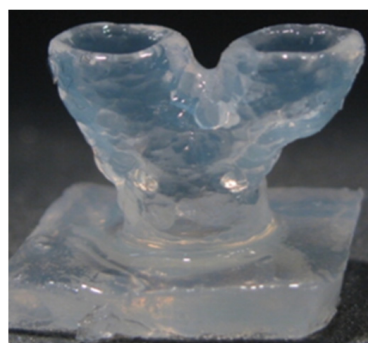
Figure 8. Self-standing arterial bifurcation model. Reproduced from Andreas Blaeser et al. [29].
