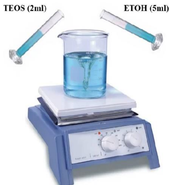
Figure 1. Synthesis method of \text{SiO}_2 nanoparticles.
