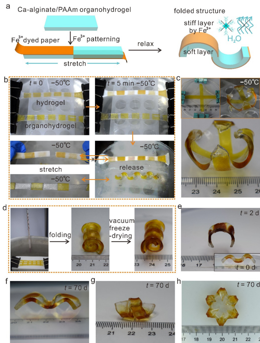
Figure 1. Shape morphing of Fe (III)-patterned tough organohydrogels at -50\text{ }^{\circ}\text{C} and long-term storage under arid conditions. (a) Scheme of the shape morphing process enabled by the paper transfer patterning of Fe(III) ion aqueous solution on a pre-stretched tough organohydrogel. (b) Pre-stretched patterned gels (organohydrogel and hydrogel) were subjected to a temperature of -50\text{ }^{\circ}\text{C} . After release of the tensile strain, the organohydrogel folded into a sinuous line, while the frozen hydrogel remained in its stretched shape. (c) A more complex folded flower shape realized at -50\text{ }^{\circ}\text{C} . (d) Illustration of the high drying tolerance of the organohydrogel under vacuum freeze-drying conditions. (e) Dried hydrogel after exposure to an arid environment (50% humidity) for 2 days. (f–h) Soft organohydrogels after exposure to an arid environment (50% humidity) for 70 days: (f) sinuous line shape, (g) spiral shape, and (h) flower shape.
