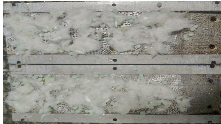
Figure 8. Distribution of the temporary plugging materials in a simulated fracture.
