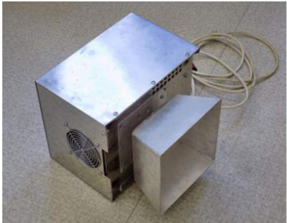
Figure 2. Examining power generator with horn antenna [25].
