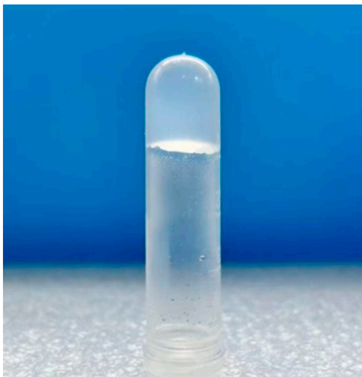
Figure S5. The gelation of hydrogel was activated by the nanoclay without BIS.
