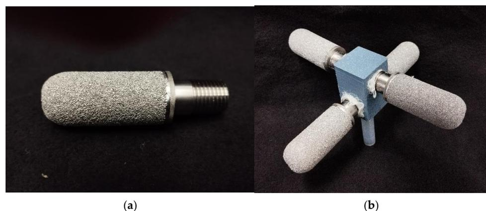
**Figure 4.** (a) The porous pin disperser ( $50 \mu\text{m}$ ) influenced the development of the bracket design through its significant length. (b) Shows the assembled disperser, which prevents any contact with
