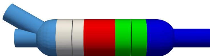
**Figure 12.** Geometry of the mixer with reduced length and number of baffles.
