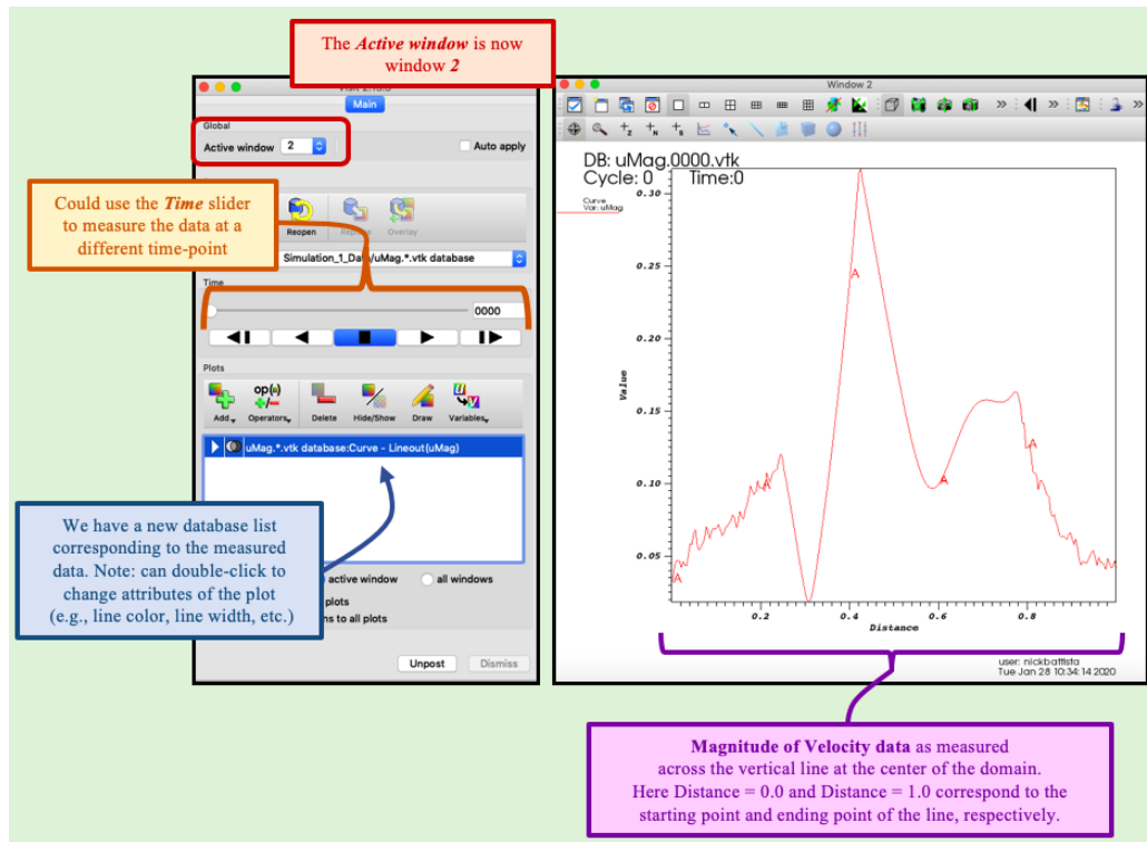
Figure 18. Illustrating the Active window change to window 2 as well as a plot of the magnitude of velocity (selected data) as measured across a vertical line at the center of the domain.
