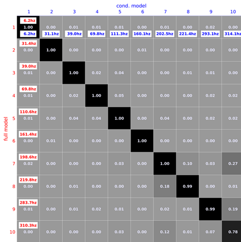
Figure 11. Modal assurance criterion (MAC) matrix of full and condensed model.
