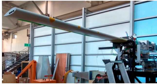
Figure 19. Model mounted on test stand outside the tunnel.
