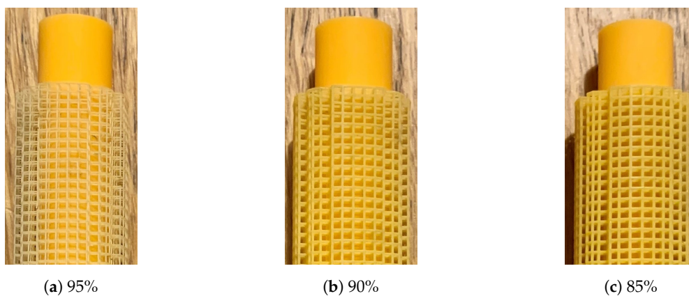
Figure 4. Porous coatings with constant lattice size and variable porosity.
