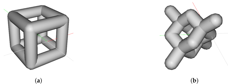
Figure 3. (a) Cubic cell; (b) diamond cubic cell of lattice size = (1.5)^3 \text{ mm}^3 and lattice thickness = 0.5 mm.
