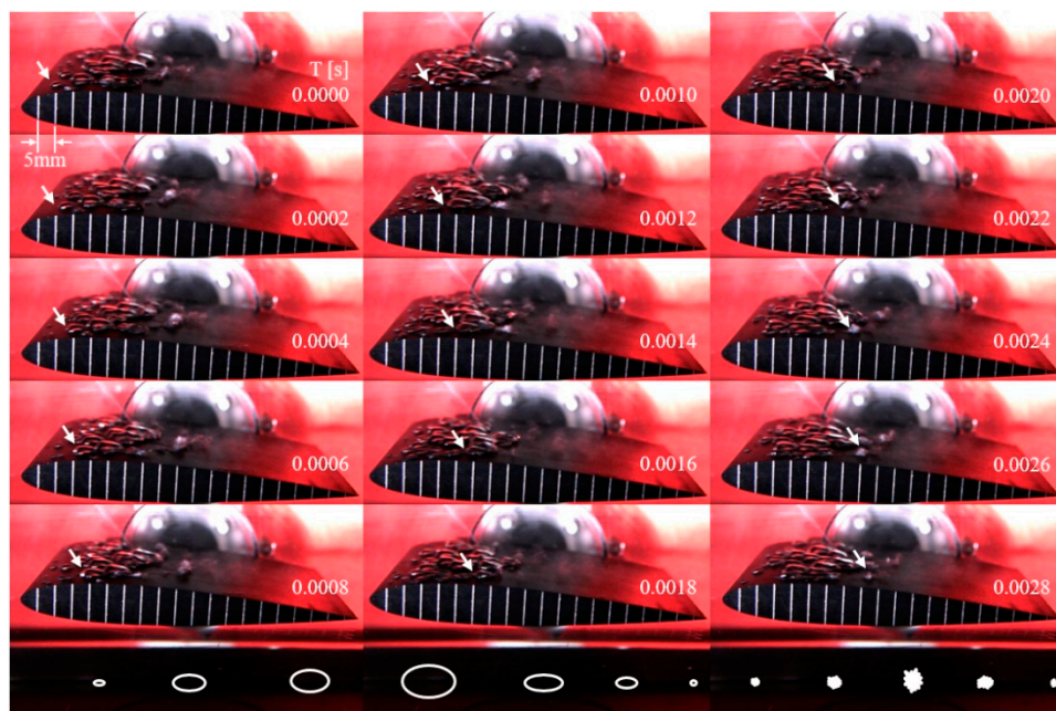
Figure 8. Evolution of bubble cavitation and collapse ( \alpha = 3^\circ , \sigma = 1.00 ).
