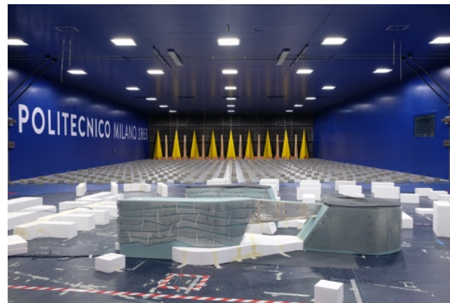
Figure 3. Wind tunnel tests on 1:75 scaled model of the ENI Head Office buildings.
