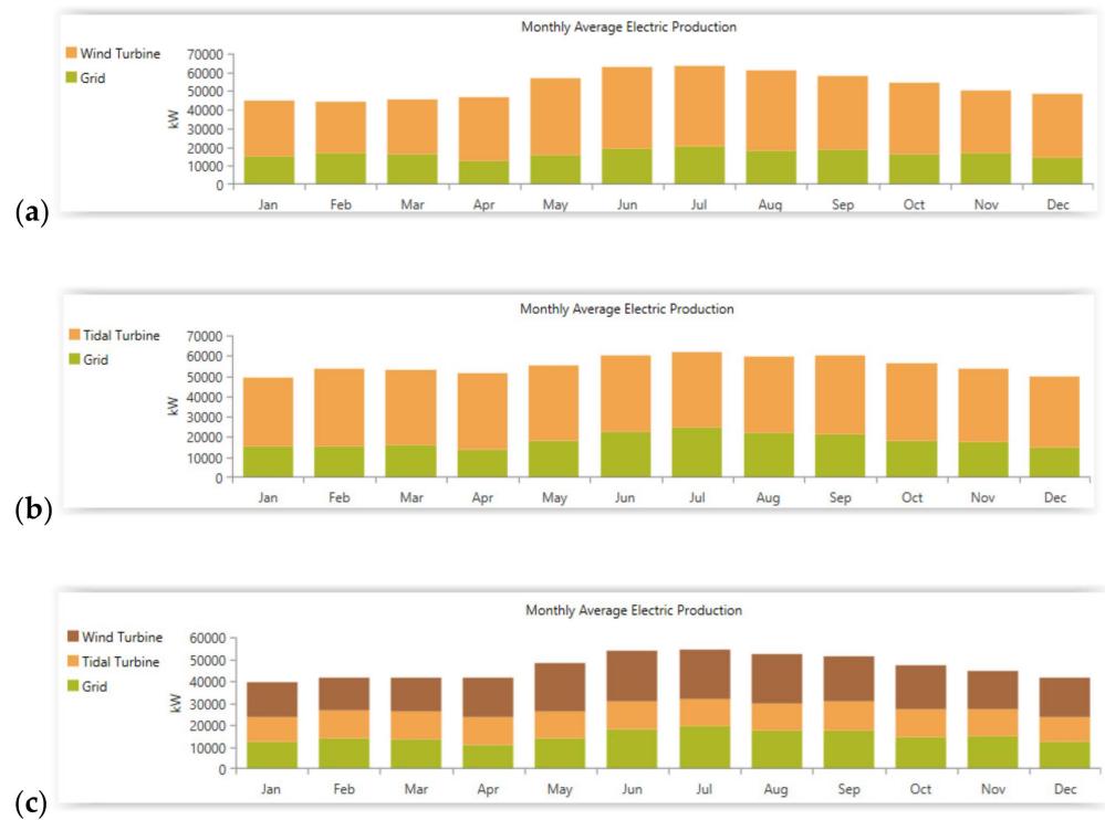
Figure 18. Monthly average output power for (a) 36 W, (b) 113 T, (c) 19 W + 38 T.
