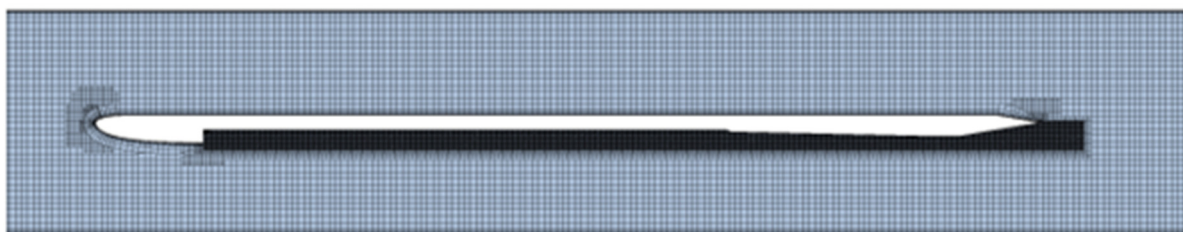
Figure 4. Numerical mesh in the fluid domain.
