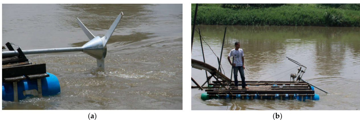
Figure 1. Photographs of the Aquavatio turbine: (a) detail of the rotor with hub and blades; (b) barge with the turbine in operation in the Cauca River; notice the axis inclination angle. (Images courtesy of Aprotect).
