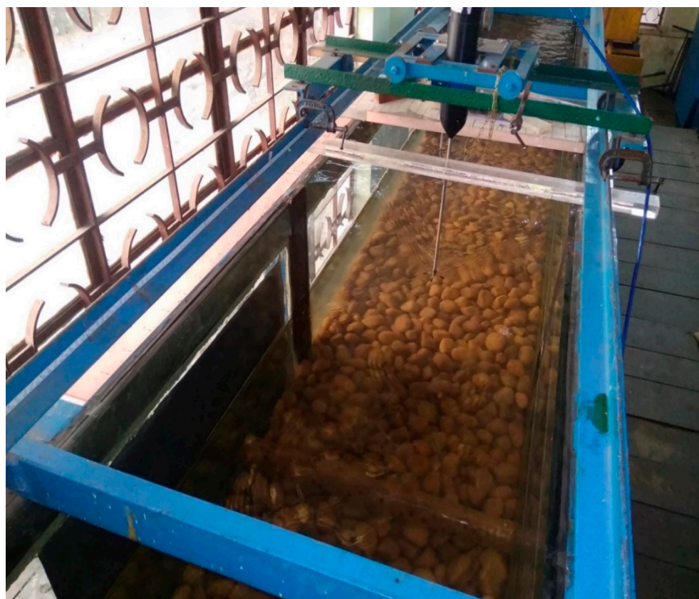
Figure 3. The flume setup for the gravel-bed (GB 1).
