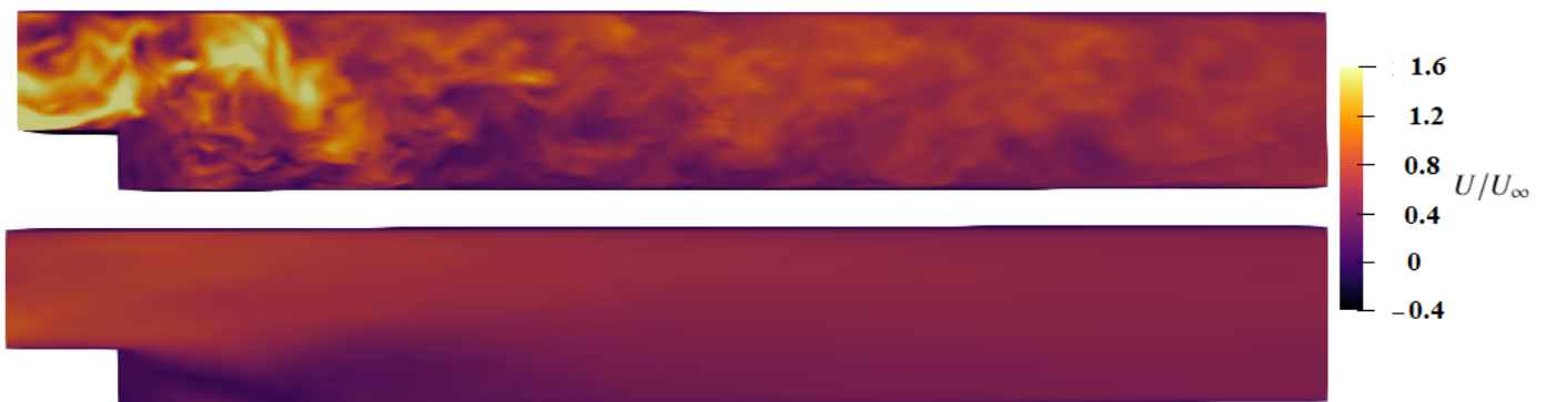
Figure 9. The instantaneous (upper) and mean velocity (lower) in the isothermal wall configuration.
