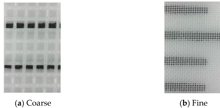
Figure 1. Samples of the two wire mesh screens used in the bubble point test; (a) coarse and (b) fine. The black bars in the background belong to a millimeter scale.
