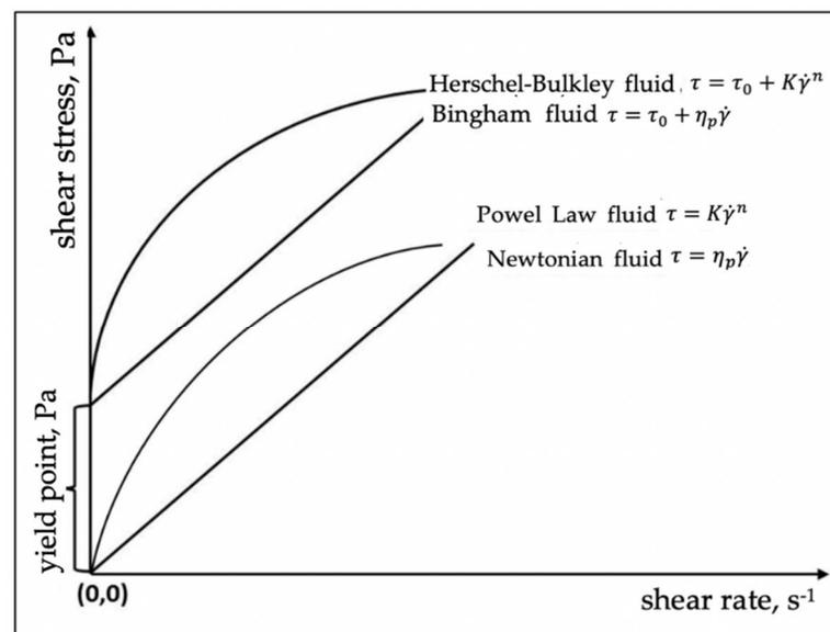
**Figure 1.** Flow curves of fluids obeying different flow models.
