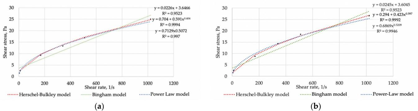
**Figure 5.** Selection of the rheological model for sample 4 with PHPA MM = 20 million (a) and for sample 5 with PHPA MM = 27 million (b).
