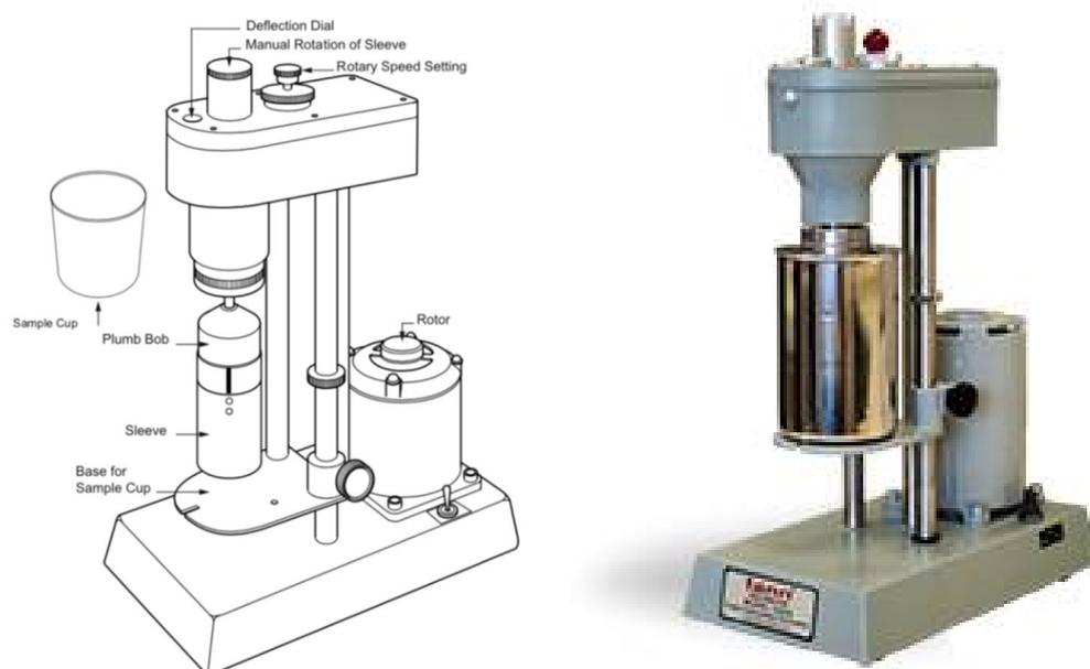
**Figure 2.** Fann rotary viscometer.
