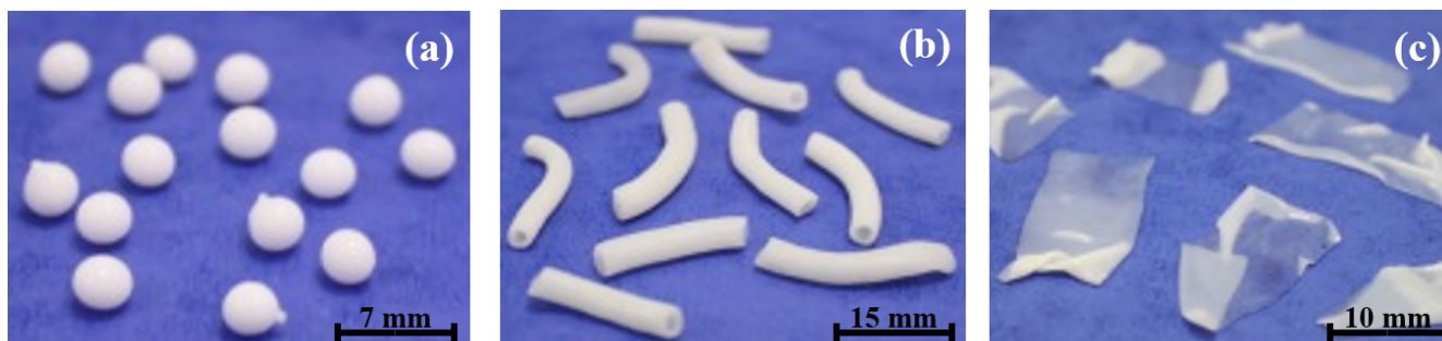
Figure 1. Photographs of media used in the study: (a) beads, (b) hollow cylinders, and (c) sheets.
