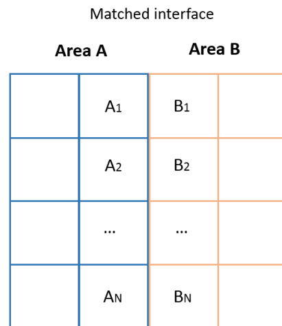
Figure 2. Schematic example of a grid with a matched interface.
