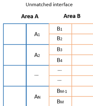
Figure 6. Schematic example of a grid with an unmatched interface.
