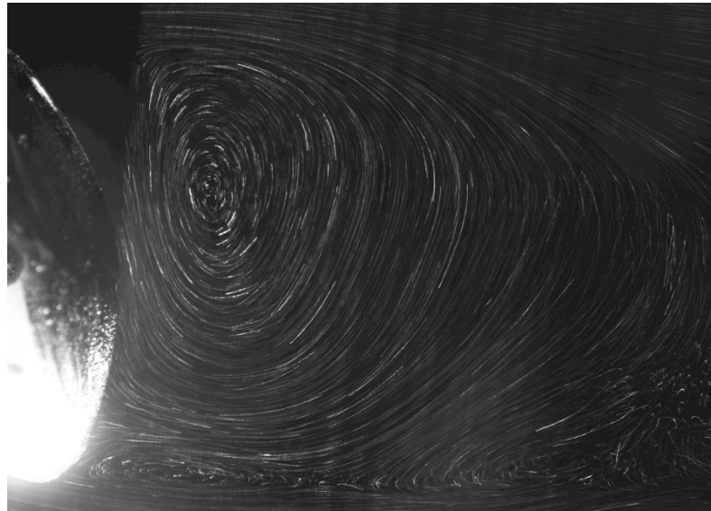
Figure 5. This experimental figure shows a two-dimensional slice of the wake vortex structure formed behind a spheroidal body. The wake is illuminated using a laser sheet, which is scattered by the micron-sized glass powder, which seeds the fluid, thereby illuminating and revealing the vortex spiral. This can be thought of as a zoomed-in image of the computational wake image shown in Figure 4.
