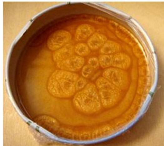
Figure 2. Benard convection cells observed in gold paint heated from below. Image taken from [43].
