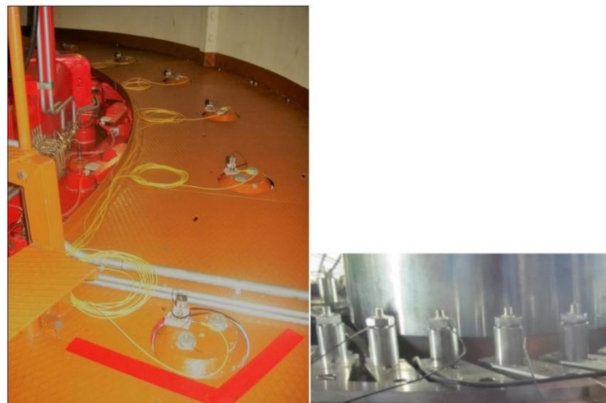
**Figure 2.** Vibro-acoustical sensors on the guide-vane trunnions.
