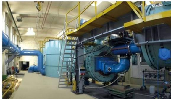
**Figure 1.** One of the five model-test rigs in the Andritz Hydro Laboratory in Linz, Austria.
